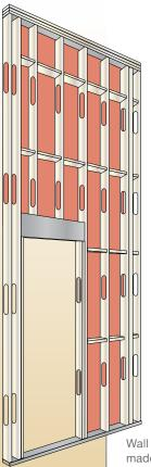
Wall panels can be made from wood or steel studs, whichever the project calls for.
